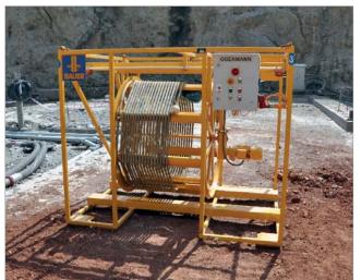
Inclinometer drum, equipped with SAA scan
