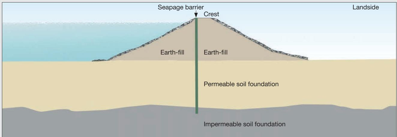
Seepage, piping, partial liquefaction, surface erosion due to flooding or wave action, usually cause significant damage to the protection system. With the appropriate product, such as a cut-off wall, this can be prevented or significantly mitigated.
