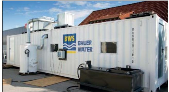
Our cleaning method removes contamination, using precisely engineered ultra-high pressure water jetting technology. Water is recycled within the water treatment system for reuse in the subsequent decontamination processes, which in turn minimizes the volume of secondary waste. Both, inside and outside cleaning are applied in the decontamination cabinet. NORM clearance measurements and quality checks are executed in a controlled "clearance" container.
