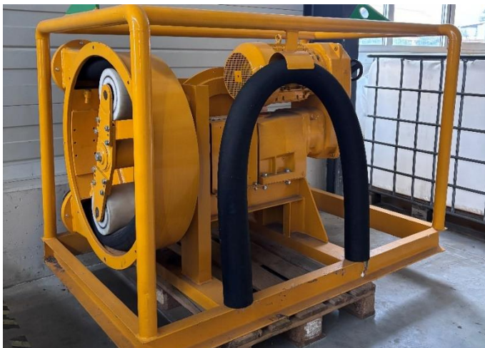
(3) Prototype of an SP 800 hose pump (1994/95)
