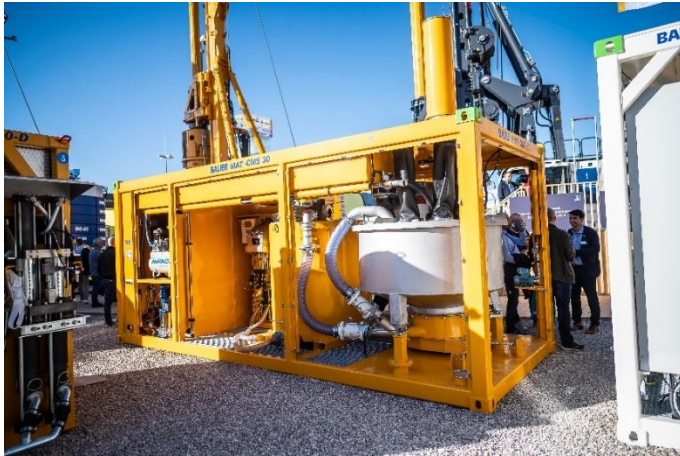
(4) Batch Mixing Plant CMS 30 with integrated Grouting Pump DP 101
