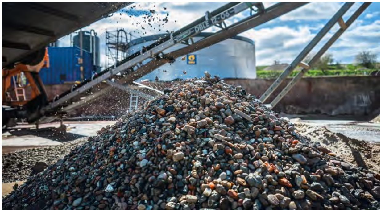
The mobile soil washing plant combats PFAS contamination.
