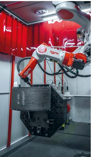
In the 10 x 10 m robotic cell, construction components can be welded with a length of up to 2 m and a weight of up to 2 t (top), while the welding robot is programmed and controlled by tablet (right).
