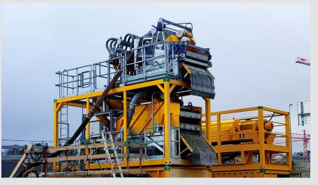
**Netherlands** For a new attraction on the coast of the North Sea, the company BodemBouw B.V. used an RTG RG 21 T for the execution of a CSM wall. **bottom**
