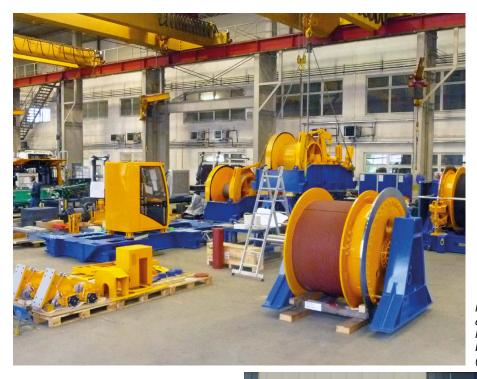
In the manufacturing hall, the individual components are assembled to form hoists (left). The hoist SBN FH-55 can be transported using a modular trailer (bottom).
