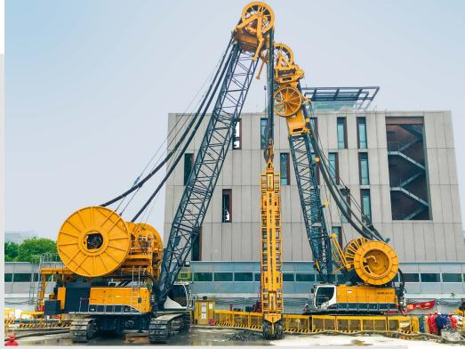
**China** Shanghai Tunnel Engineering Co. Ltd. used a BC 40 cutter on a MC 96 dutycycle crane, as well as a BC 50 cutter on a MC 128 duty-cycle crane, in the Chinese metropolis of Shanghai. **top**
