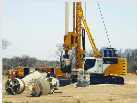
**USA** Bauer Equipment America carried out various test runs on the company premises in Conroe, Texas, with a BG 33 using the Kelly drilling method. **bottom**
