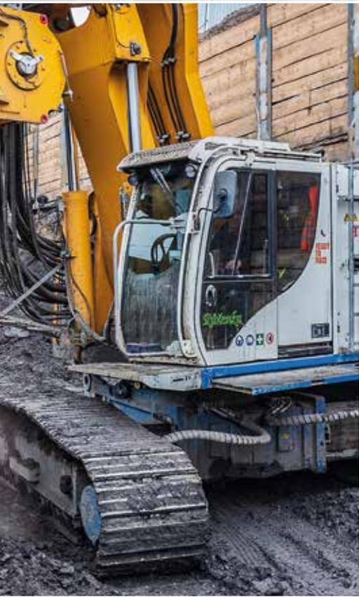
**Italy** In the city center of Padua, our customer Impresa Marini Ermenegildo S.p.A. used a BG 39 with a cased continuous flight auger. **Bottom**
