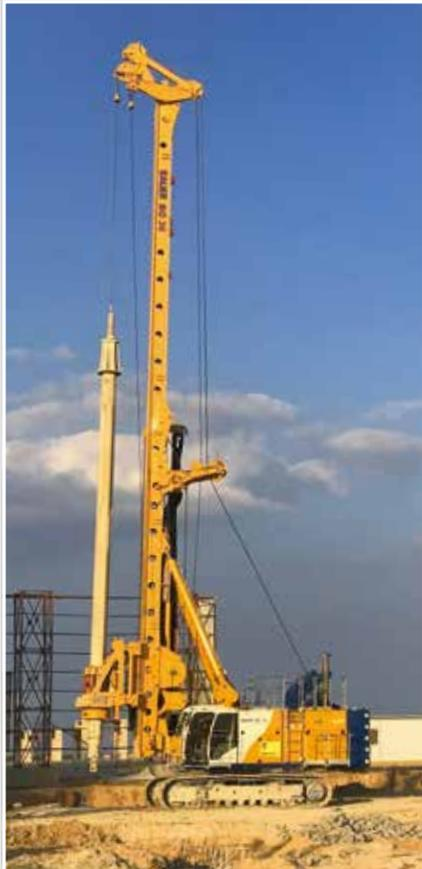
**Egypt** Our customer Arab Contractors Mechanical & Electrical Engineering drilled foundation piles down to a depth of 30 m, using a BG 36 V in Kelly drilling mode. **Top**
