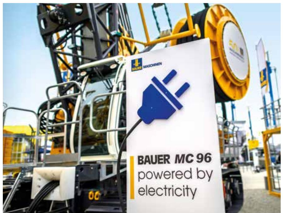
ward putting an idea into practice and unveiled its first electrically driven cutter at Bauma. The cutter is based on a BAUER MC 96 duty-cycle crane and is equipped with a powerful 500 kW electric drive.
