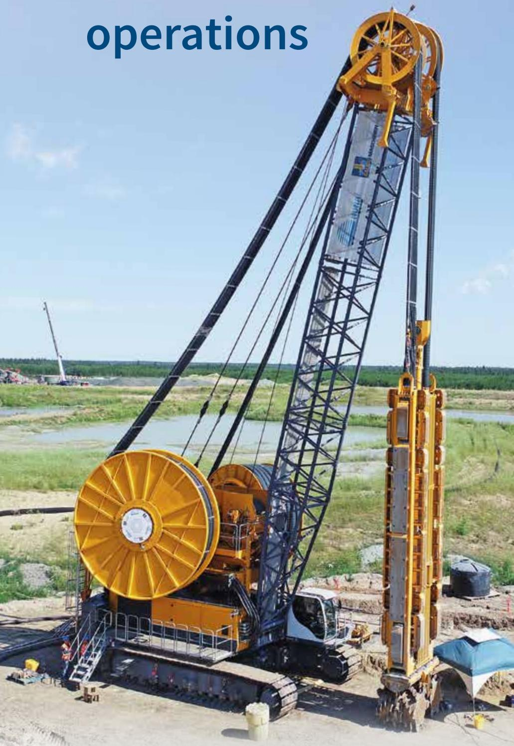
**Canada** As part of the FalCon project in Saskatchewan, samples were taken successfully at a cutting depth of 251.4 m. Prior to this, no other cutters worldwide had reached this depth in commercial applications. The FalCon project by Rio Tinto Exploration Canada Inc. and Star Diamond Corporation, aims to demonstrate the geological viability of the kimberlite fields at Fort à la Corne. A BC 50 cutter and an MC 128 duty-cycle crane were used for sampling. **Top**
