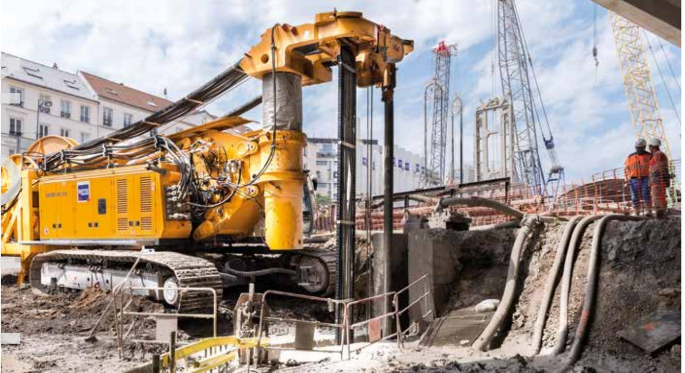
*MC 64 with low-headroom trench cutter for construction of an underground parking garage in Paris.*
