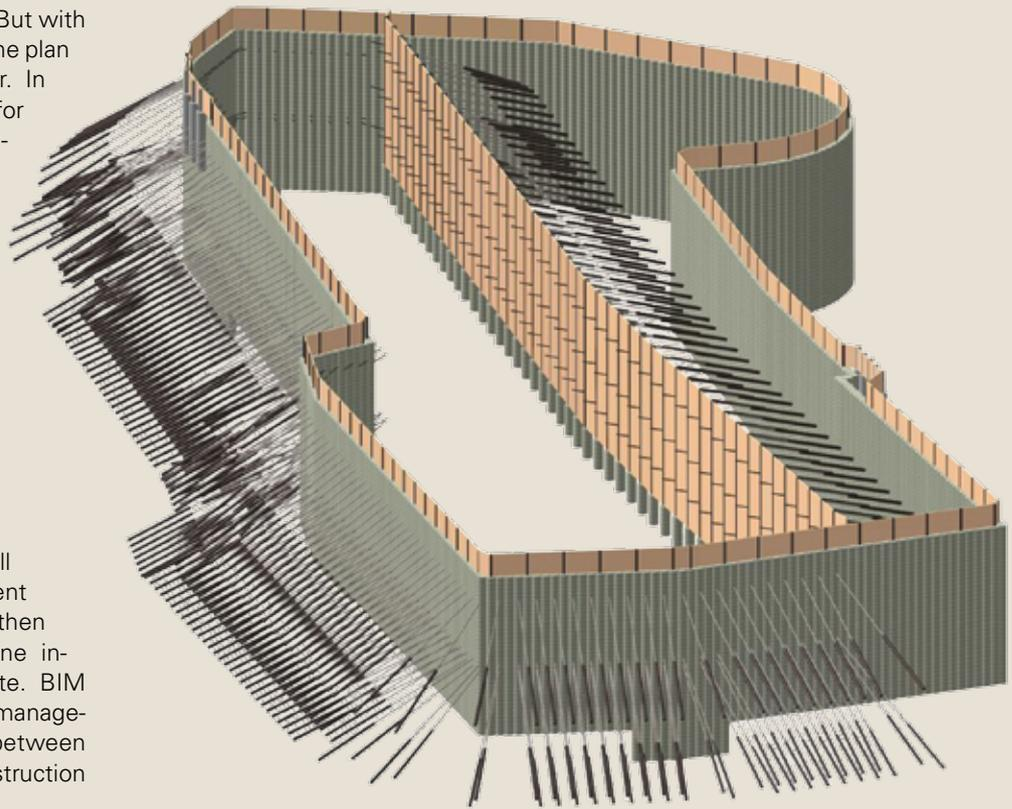
*3D model of an excavation pit with pile wall tied back with anchors.*
