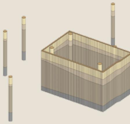
*Derivation of soil stratification and excavation quantities in the CAD system.*
