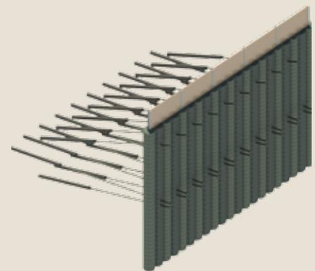
*Part of a model: pile wall with I-beam shoring and anchor layers.*
