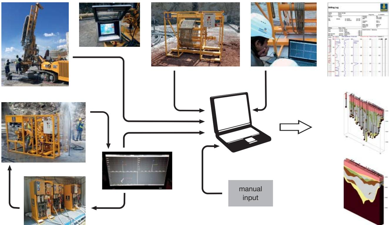
Schema of grouting data collection system
