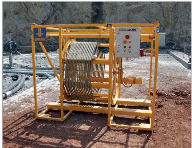
Inclinometer drum, equipped with SAA scan
