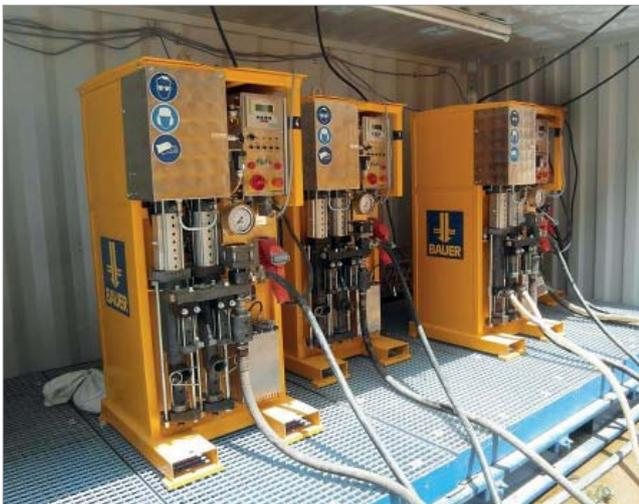
Hydraulic controlled grouting pumps in container
