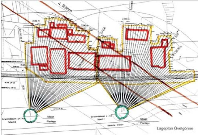
Compensation grouting from 5 shafts at Elbtunnel Hamburg
